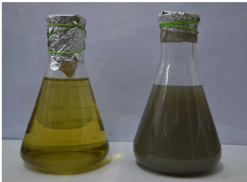
Figure 2: Change of color from yellowish to brownish after adding 1mM \text{AgNO}_3 to the ipomoea pes-caprae leaf extract
